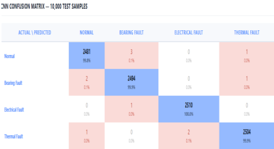
Graph 11: CNN Confusion Matrix — 10,000 Test Samples
