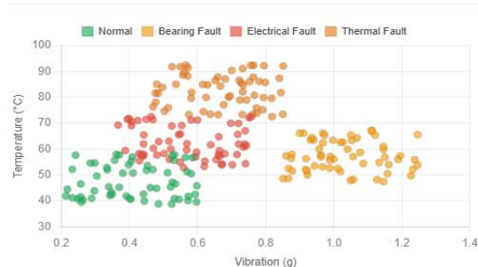
Graph 28: Vibration vs Temperature — by Fault Type
