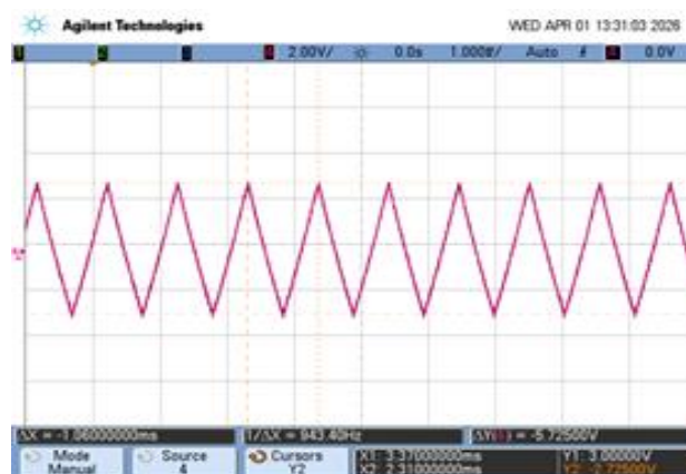
Fig.2(c) Triangular waveform.
