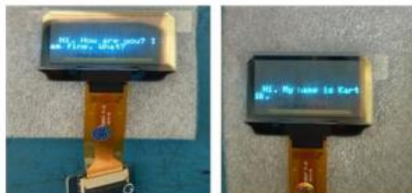
Figure 7. T-OLED display showing the recognized speech converted into text and displayed as subtitles
