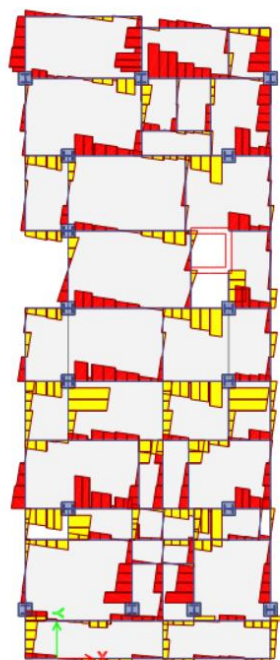
Figure1.11: Shear Force Diagram
