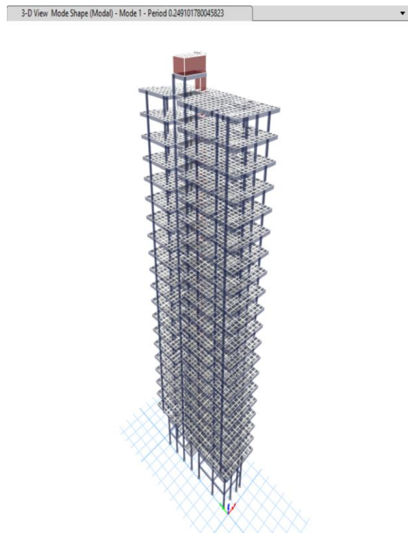
Figure1.8: Model View for Mode Shape-1
