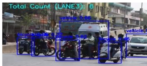
Fig. 5(c) Display Output depicting vehicle detection and counting - Lane 3
