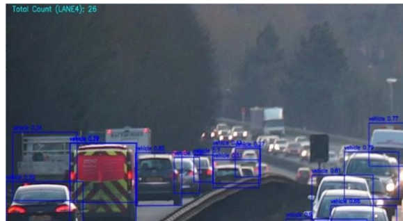
Fig. 5(d) Display Output depicting vehicle detection and counting - Lane 4
