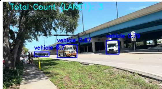
Fig. 5(a) Display Output depicting vehicle detection and counting - Lane 1
