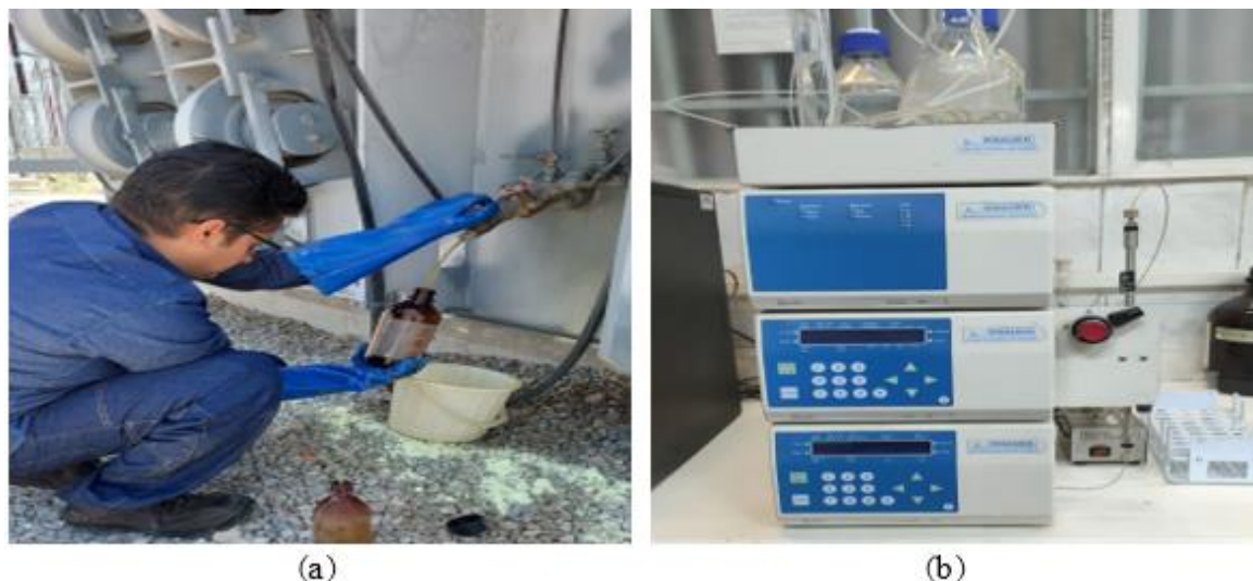
Figure 3: (a) Oil sampling from T3. (b) HPLC for measurement of oil-soluble furfural.
