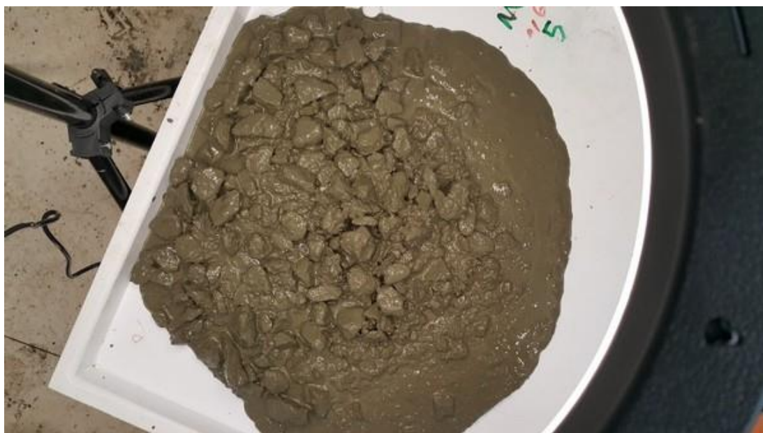
Figure 1. Freshly mixed concrete photographed under the standardized smartphone image-acquisition setup.
