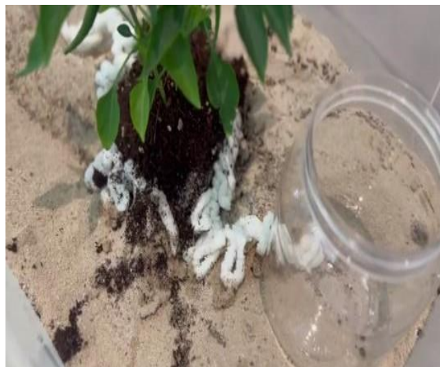
Fig. 3. Green Desert prototype demonstrating Wick-Based Irrigation Mechanism
